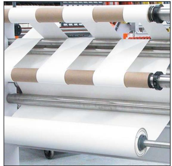
Slit strips are alternately rewound on the two removable rewind shafts, preventing interleaving.
